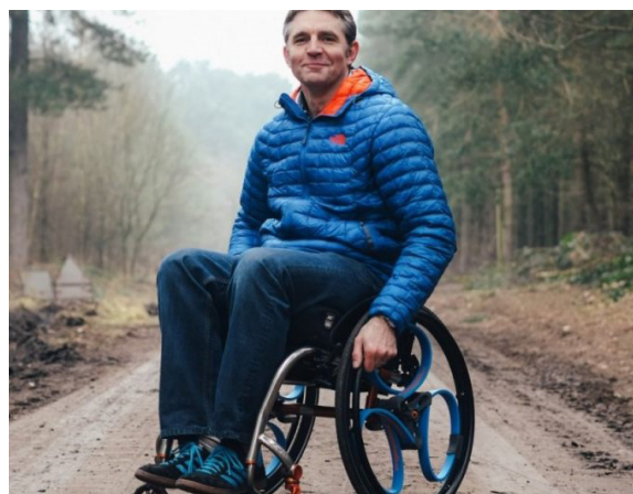
The TECHNIA Simulation Centre of Excellence has worked together with Loopwheels on development of vibration-reducing wheels, which offer significantly improved wheelchair performance. Compared with a traditional spoked wheel, vibrations are reduced by up to 70 per cent, giving users of Loopwheels' wheelchairs better comfort and a softer ride.
